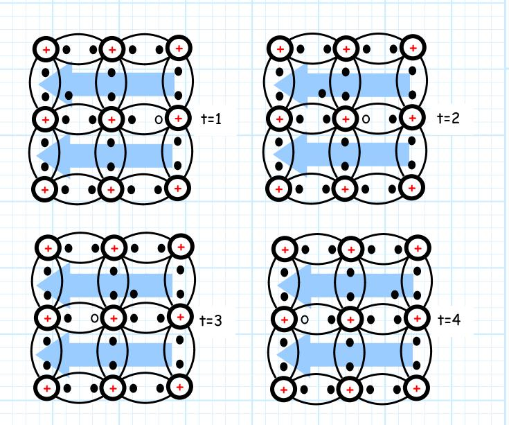
\* Note over time, the **free electrons** move from **left to right**, in response to the electric field.
